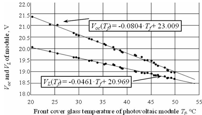
Fig. 2 Dependency between values of open circuit voltage  $V_{oc}$ /voltage under optimal load  $V_L$  of photovoltaic module and the front cover glass temperature  $T_f$ , determined based on experimental data set and algorithm (12). The values of  $V_{oc}$  and  $V_L$  for standart test conditions temperature ( $25^\circ\text{C}$ ) are 21 V and 19.8 V, respectively
