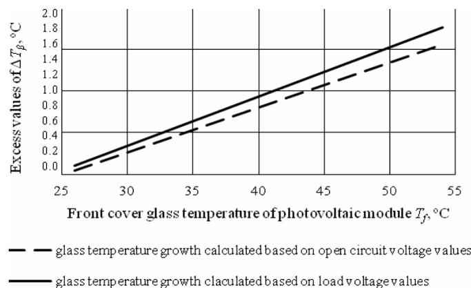
Fig. 3 Excessive values of front glass cover temperature of external module surface  $\Delta T_f$  over  $T_f$  temperature for two modes of work: without external load (dashed line) and with external load connected (solid line)
